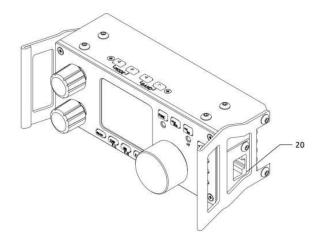
**20 MIC Interface** (On the right side of the machine-head) Connecting the multi-function MIC to this connector.
